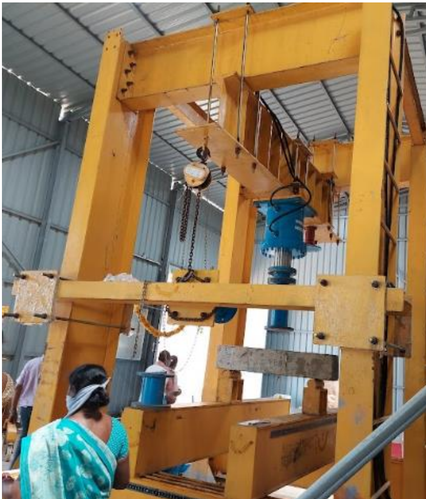
Loading Frame-Facility (200T Transverse, 20T Lateral)
